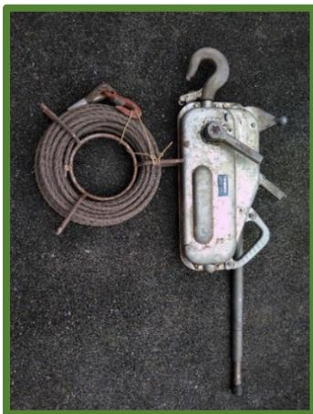
**Grip hoist:** A portable manual hoist with wire rope that can lift, pull, and move heavy loads across great distances (figure 7.0.10).
