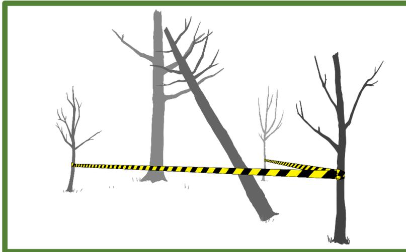
**Figure 7.0.1—Flagging off a hung-up tree.**
