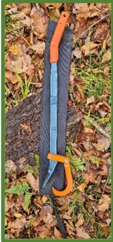
**Felling lever:** A multitool made to replace wedges that can provide lift during felling and roll logs during bucking (figure 7.0.8).
