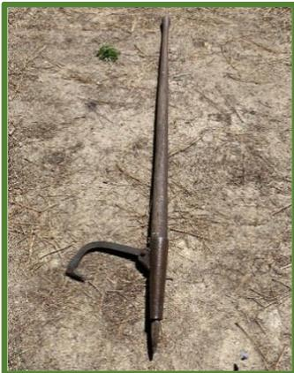
**Peavey:** A forester's lever with a pivoting, hooked arm and a metal spike at one end (figure 7.0.9).
