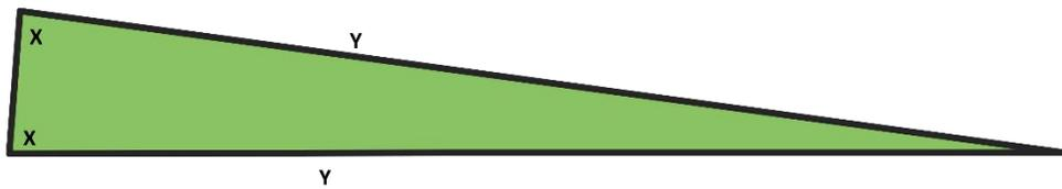
Figure 6.0.3—A double-taper wedge is an isosceles triangle with two equal sides.
