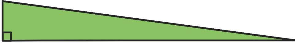
Figure 6.0.2—A single-taper wedge is a right triangle with a 90-degree angle on the back plate and three unequal sides.
