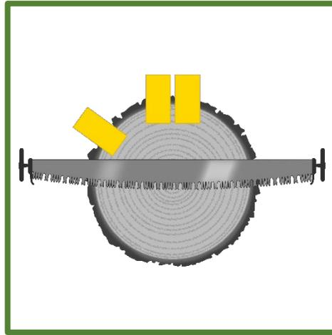
**Figure 6.0.10—Wedging technique top bind and side bind.**
