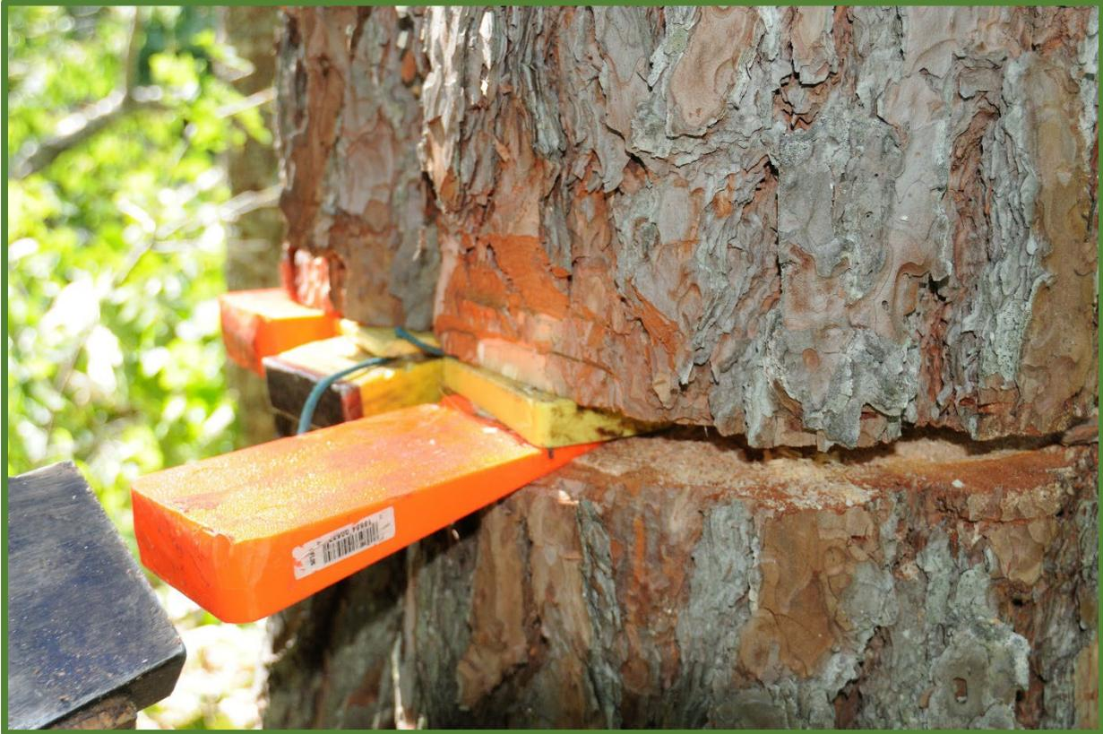
**Figure 6.0.14—Combining shims with a standard wedge.**
