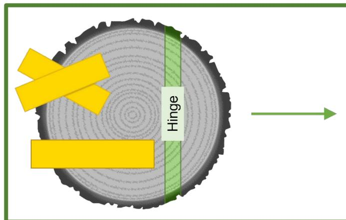
Figure 6.0.13—Crossing/stacking wedges.
