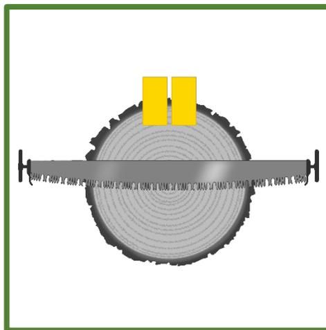
Figure 6.0.9—Wedging technique for top bind.
