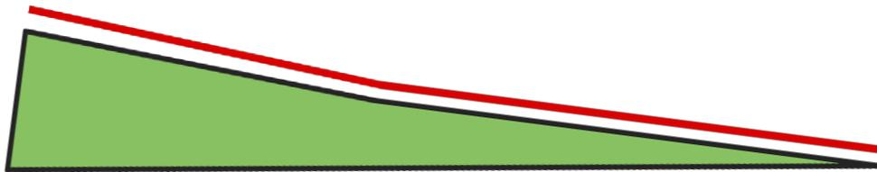
Figure 6.0.4—A triple-taper wedge starts similar to the single-taper wedge, but steps up the degree of incline about half-way into the taper.
