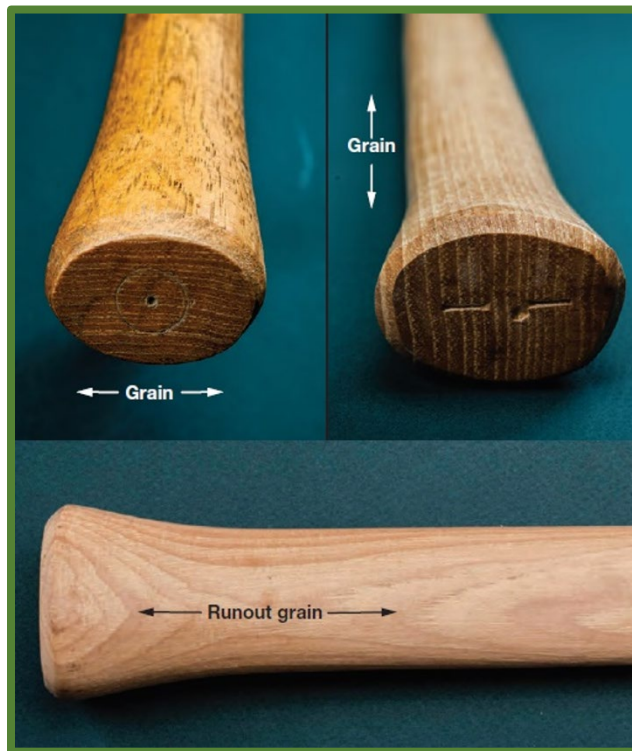
Figure 4.0.5—Wood grain examples.
