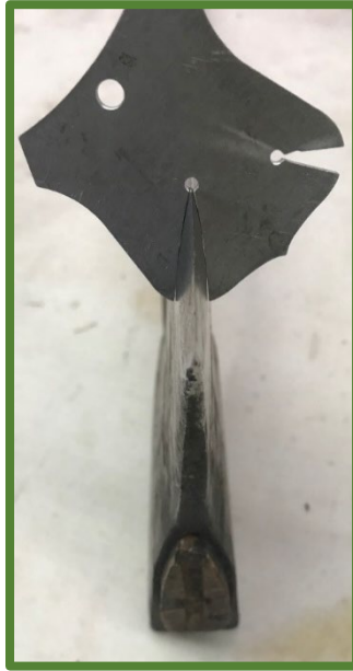
Figure 4.0.7—A cheek gauge showing a correctly profiled ax.
