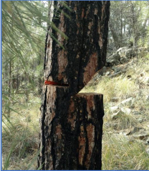
Sawyers view of buried wedge and hinge wood.
