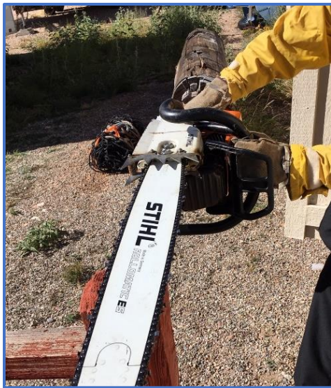
Hand position that WOULD activate chain brake during reactive force or kickback.
