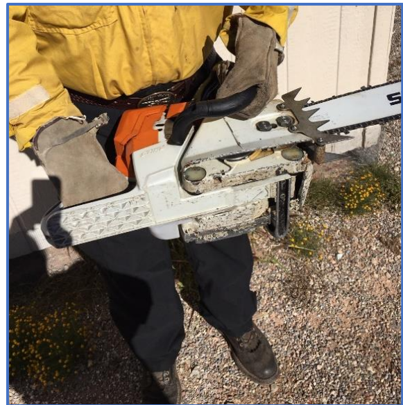
Hand position that would NOT activate the chain brake during reactive force or kickback, as was the case in this incident
